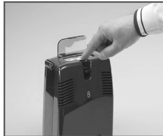
Figure 17: Pressing Flow Selection Button
